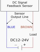
DC signal feedback device External circuit diagram
